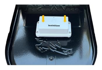
Press both ends of the sensor firmly so that the two Velcro strips fasten securely.
